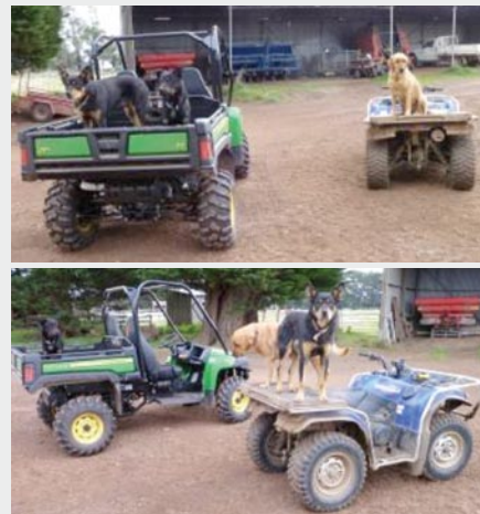
Side by side vehicles (shown above left) have a longer and wider wheel base and are more stable than a quad bike. They also have a roll over protection device and most are fitted with seat belts. Side by side vehicles may be a safer option for many jobs around the farm
